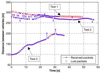
Figure 5. Distance between the two vehicles for the car-following communications assessment tests
