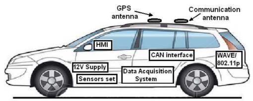
Figure 4. Schematic of a vehicle instrumented with an OBU Cooperative ITS prototype
